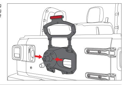
3. Using T25 Torx drive, remove seven screws securing cover plate to third brake light mount.
