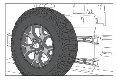
2. Using T25 Torx drive, remove two screws securing lug stud assembly to factory tire carrier. Remove lug stud assembly, including back up camera, and set aside for later use.
