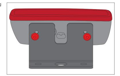
12. Plug in third brake light and attach assembly to supplied Lug Nuts using remaining M8 hardware and 5mm Hex Key.
