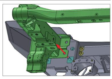
6. With bumper in place thread the hardware to the bumper. On the inside upper location it takes M12 bolt with flat and lock washer. The other three mounts use M12 nut with flat and lock washer. Do not tighten at this time just hand tighten to hold bumper in place.
