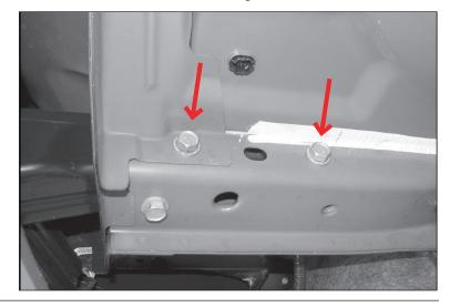
2. Bolt the Frame Mounting Bracket to frame rail with the factory 14mm hex bolts, (Figure 2). Do not fully tighten. Repeat for passenger side.
