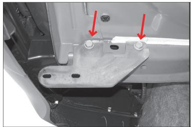
3. Carefully position Rear Bumper Guard to inside of Mounting Brackets. Bolt Rear Bumper Guard to Brackets using 12mm x 35mm Hex Bolts, 12mm Flat Washers, 12mm Lock Washers, and 12mm Hex Nuts. Do not tighten hardware at this time.
