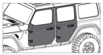
2. Loosely install Hinge Pins on Tube Doors using supplied M8 hardware.
