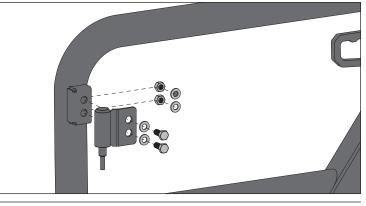
3. Using caution, slowly insert Tube Door in door hinges and reinstall factory door nuts.
