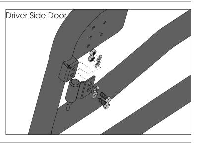
3. Using caution, slowly insert Tube Door in door hinges and reinstall factory door nuts.
