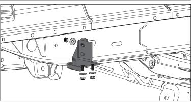
3. Remove two M10 nuts from body mount in front of rear wheel. Loosely install Rocker Guard on studs using factory M10 nuts.
