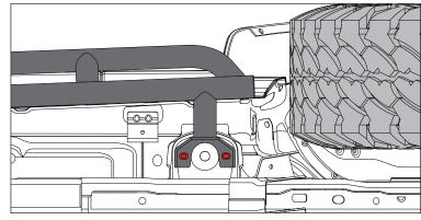
4. Attach Rocker Guard to Mounting Bracket using supplied M10 hardware. Once attached, tighten all mounting hardware.
