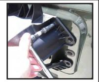
Step 3. Install the CB Antenna Mount using the supplied hex bolts, lock washers, flat washers. Torque bolts to 10 ft-lbs. Remount the spare tire after CB Antenna installation is complete.
