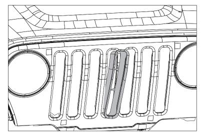
3. Press lower retainers into grille shell and press top of insert until clipped into place.
