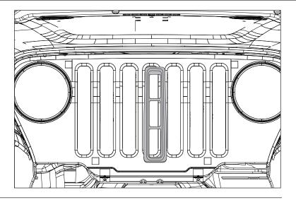
2. Insert lower portion of insert into grille opening.
