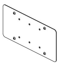
Attach Hawse Fairlead License Plate Holder to Hawse fairlead by aligning the 3 snap fittings with the opening in the fairlead. Route <u>winch</u> line between the snap fittings and push the plate evenly until fittings engage. Use supplied License Plate Mounting Bolts to attach license plate.
