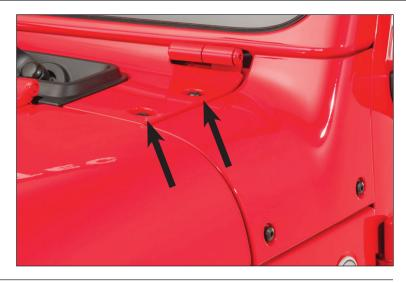
2. To install the LED mount bracket place the thicker 2.8mm stainless washer in front cowl location and the thinner 1.5mm stainless washer in the rear cowl position. Now place the plastic spacers on top of the stainless washers. Place bracket on top of the spacers and feed the Button head bolt and washer (provided) through the bracket and spacer to the threaded hole. Tighten to secure, **DO NOT over tighten or use power tools to tighten**.
