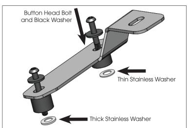
3. To install two pairs of cubes simply stack the 11232.72 inside bracket and 11232.73 outside bracket. The 11232.72 inside mount bracket will mount towards the bottom and the 11232.73 outside mount on top. With this order it allows the LED light tabs to be level with each other. Use the same hardware and plastic spacers to mount the double brackets.
