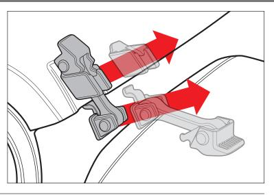
2. Using supplied M8 flat head bolt and nut, loosely attach locking latch assembly and fender gasket to OE fender.
