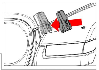
3. Using supplied M6 flat head bolt and nut, loosely attach hood mount and hood gasket to the vehicle.
