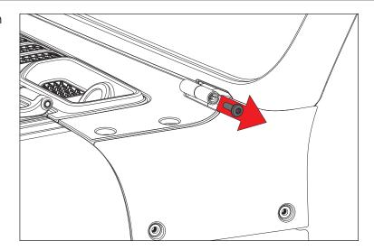
2. Loosely install M12 Jam Nut and Mirror Arm on Mounting Stud.
