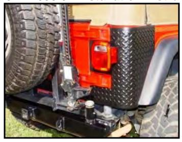
**Step 1:** Remove both left and right side rear taillight assembles. This will require the removal of 3 bolts for each light that are assessable from the inside of the tail light assembly and from the upper inside of the fender. The lower plastic fender cover can be pulled back without removing. The left side license plate holder and fuel filler neck will also be removed.
