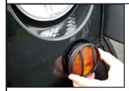
**Step 7.** Re-insert the housing into the grille. Push the housing back until it snaps into place.
