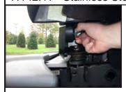
**Step 1.** Begin by removing the bulb and socket assembly from the marker light. Twist the socket up and away from the vehicle until it loosens.
