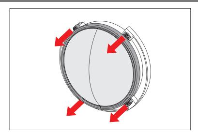
5. <u>Install Pivitol Headlight Guard</u> using factory screws in one of three configurations, vertical, horizontal, or diagonal. Each guard will work for both headlights.
