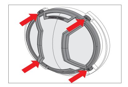
6. <u>Reinstall grille and turn signal</u>, see steps 1 through step 4.
