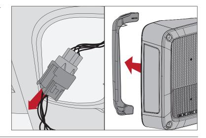
3. <u>Encase tail light inside Housing and Guard</u> using M5 Screws.
