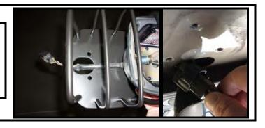
Step 9: Reinstall the tail light assembly and Euro Tail Light Guard to the original mounting holes using the factory hardware previously removed.
