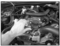
3. Disconnect the electrical connector from the bottom of the throttle body.
