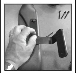
8 - Tighten mounting bracket to windshield.
