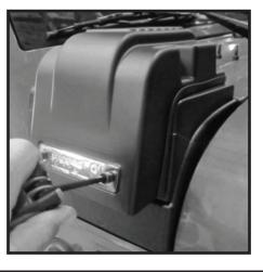
**3** - Remove low mount intake. Make sure "U" gasket is retained for future use.
