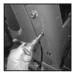
7 - Insert (4) M6 caps head bolts and washers through intake to snorkel main body. Tighten bolts.
