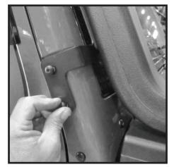
9 - Tighten mounting bracket to high intake M6 bolts. Turn on windshield wipers to check for clearance. Adjust as needed. NOTE: vehicle must be equiped with OE correct 16" wiper blades.
