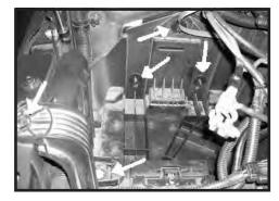
Step 3. Remove the three nuts and two bolts in the battery section of the tray.
