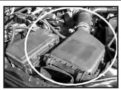
Step 2. Remove the PCV hose from the filter box.
