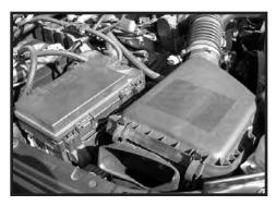
Step 16. Reinstall the battery tray, battery, power fuse box, steering reservoir and bracket, and air box. Start motor and check for exhaust leaks.
