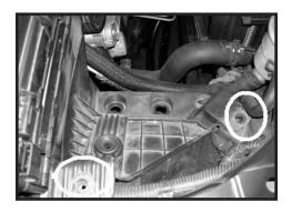
Step 6. Remove the two front tray mounting bolts.
