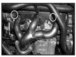
Step 12. Install the passenger side header, and gasket. Install the upper flange bolts with the exception of the top left and right bolts. These bolts will be used to hold the factory heat shield in place. Install the down pipe flange bolts on each side
