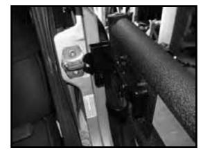
6. Attach the loop of the Adjustable Nylon Strap to the hook on the Tube Door and the hook inside the vehicle. By using different loops to attach to the vehicle hook, the amount of door opening can be adjusted.
