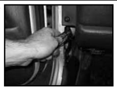
3. Remove the nuts from the bottom of each factory hinge pin. Set these nuts aside to be re-installed on the Tube Doors. To remove the factory doors, carefully lift the door upward until the hinge pins completely clear the hinges. Store OE doors in a safe place.
