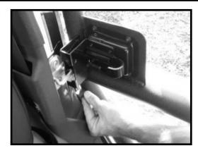
2. Drill a 3/32" hole in the Tube Door and attach the bumper with the supplied sheet metal screw. Do not overtighten. The attachment screw can be loosened or tightened as necessary to adjust the length of the Anti-Rattle Bumper.
