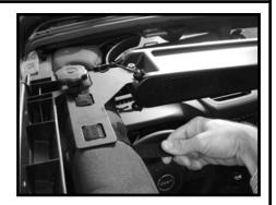
3. Insert the Short hook and loop fastener Strap through the slot in the rear of the Storage Console and attach to the footman loop of the windshield.
