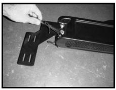
2. Place the Storage Console inside the vehicle such that the mounting brackets rest on the roll bar. The Storage Console should sit just above the visors. Insert Long hook and loop fastener Straps through the slots in each Mounting Bracket and strap them tightly around the roll bar on both sides of the vehicle.
