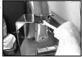
2. Install the Beam Bracket on the driver side roll bar about 3" above where the roll bar meats the body. For JK, install this bracket with the mounting flange facing upward as shown in the image. For YJ and TJ models, the bracket should be installed with the mounting flange facing downward. In all cases, be sure the U-bolt does not interfere with the seat belts, wires or roll bar covers.
