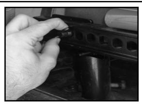
5. Adjust the bracket so that the jack is in the horizontal position. Fully tighten all nuts and wing nuts and check for interference.
