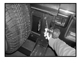
4. If installing Off Road Mounting Bracket with a RR tire carrier, secure the mounting bracket to the lower mounting plate's top two holes using M10 hardware as shown. The upper mounting plate can now be rotated into its horizontal position to line up with the mounting bracket's middle hole and the upper right tailgate hinge hole. Insert the remaining M8 hardware and tighten. Go back and make sure all bolts are tightened before inserting your Off Road Jack.
