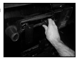
If no RR tire carrier is present, rotate the bracket installed in step 2 into its vertical position and the upper mounting plate into its horizontal position. Line up the holes in the plate and the bracket with the upper right tailgate hinge hole. Tighten the bracket into place using the remaining M8 hardware as shown. Also, fully tighten the bottom right tailgate hinge bolt.
