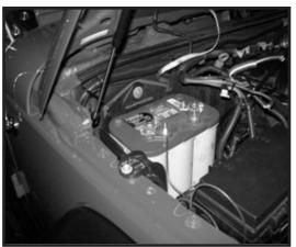
2. Remove the PVC hose from the filter box. Remove the air filter cover by unclamping the cover and removing the hose clamp on the throttle body. Remove the air filter and housing. The housing is held in by three rubber grommets on the bottom of the box. A rocking motion may be needed for removal of air box.
