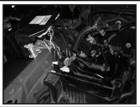
6. Remove factory battery box by removing the 3 nuts that secure the box to the fire wall and 4 bolts securing the box in the engine compartment. Save this hardware. It will be used to install the dual battery tray.
