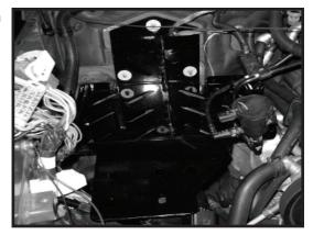
10. Check for clearance around the base of the Dual Battery Tray. Install both batteries onto tray and secure into position using supplied J-bolts and Battery strap. Slide EVAP solenoid over tab on Fuse Box Bracket. Reinstall air filter box to its original location.
