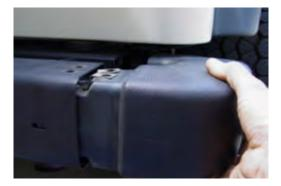
For some 97-2006 Wranglers the rear body mount and bolt may need to be removed to gain access to the top inside rear bumper bolt.
