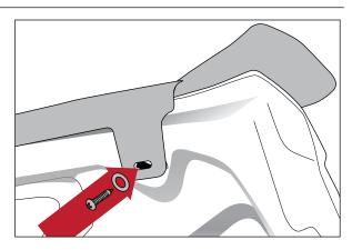
NOTE: Do not use power tools to install this product. Do not overtighten.
