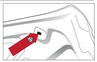
2. Remove red protective backing from double sided tape. Install bug deflector. Secure with two washers and two screws into previously plugged holes. Press firmly on taped areas and hold for 60 seconds.
