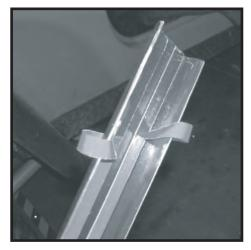
3. Carefully position Body Tub Rail Cover onto tub. Peel tape backing from one end working slowly to the opposite end. Make sure that both strips of the red protective film are being removed at the same time. Press firmly along the entire top surface after cover has been installed.
