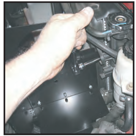
Tighten all heat shield bolts
