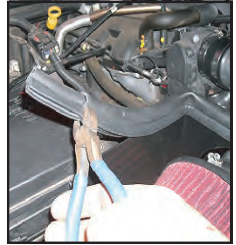
Install weather stripping
