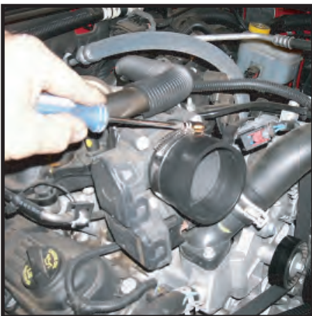
Install throttle body coupling
