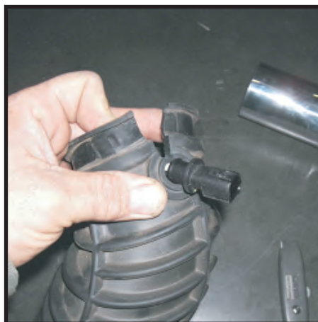
Remove temp sensor
