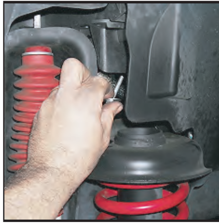
Install bolts from below
