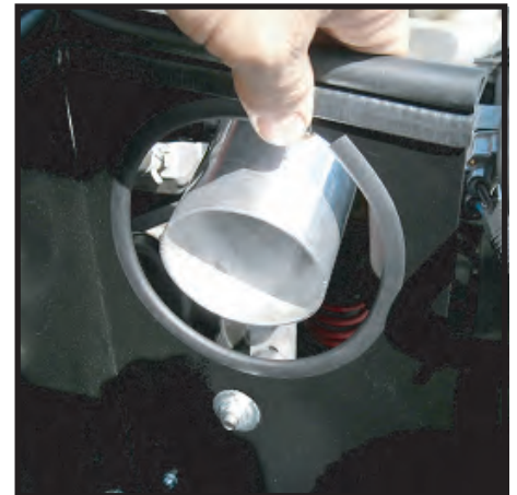
Trim secured to filter opening
