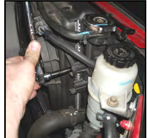
Remove upper shroud bolt
