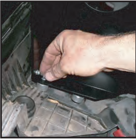
Place heat shield over spacers
