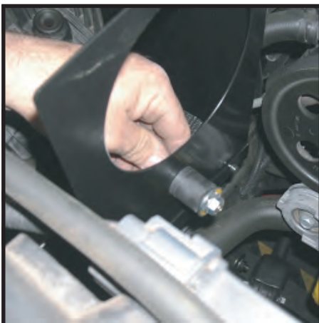
Isolator attached to heat shield
