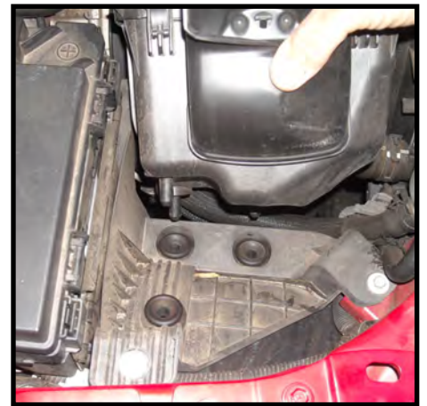
Pull air box free from inner fender
