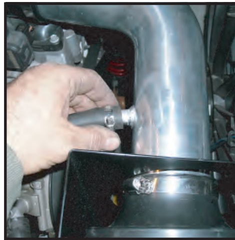
Connect breather hose with clamp
