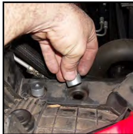
Place spacers on top of tray
