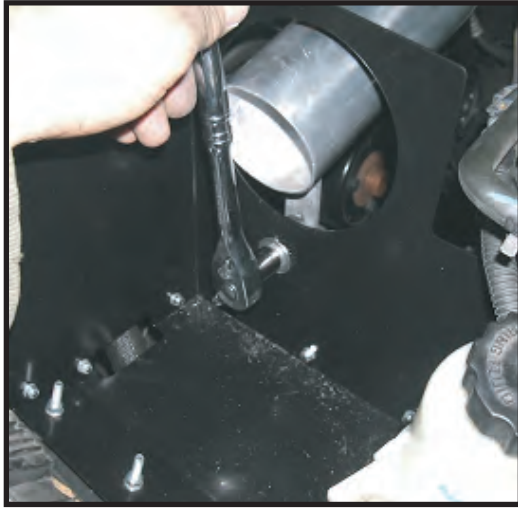
Secure tube to heat shield
