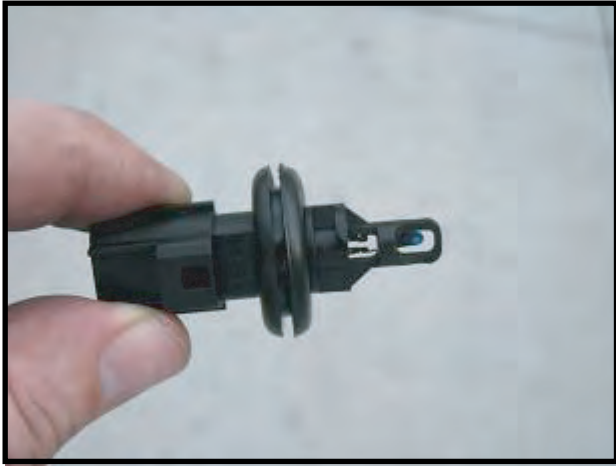
Sensor Installed in Grommet
