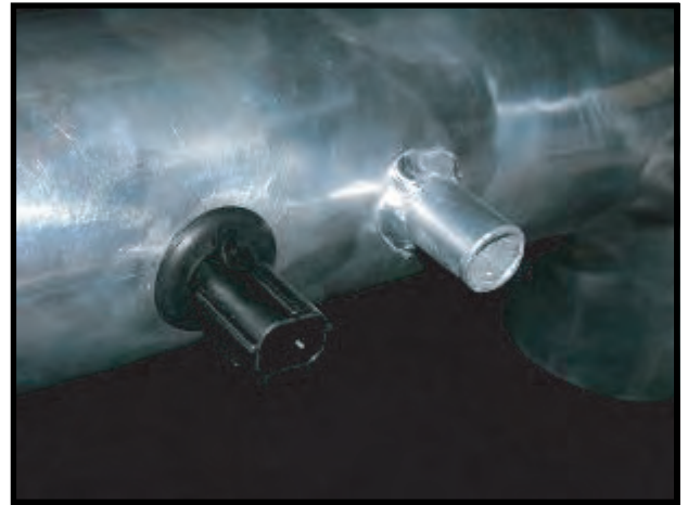
Sensor and Grommet installed in Intake Tube
