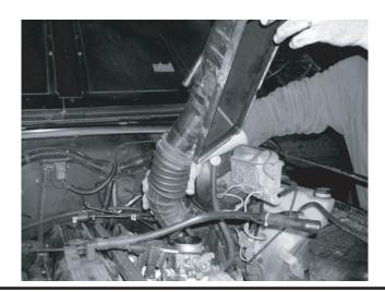
2. Mount the heat shield in place using the original mounting hardwaresaved in step 1.
