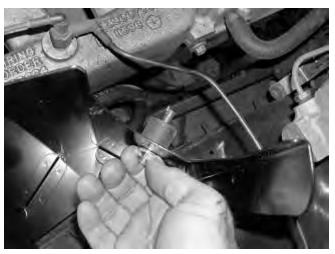
4. Install small edge trim around the intake tube area. Install the intake tube, securing with a hose clamp.
