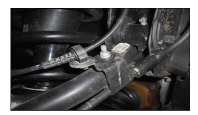
Install the brake line bracket to the control arm using M6 nut and washer. Torque to 5 ft-lbs.
