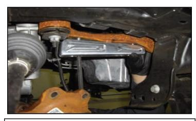
Install the provided driver side diff drop to the driver side hanger using M12 x 45mm (front) and 35mm (rear) socket head bolts. Torque to 45 ft-lbs.
