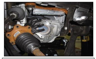
Raise the differential back into the vehicle making sure you have sufficient clearance between all components. If not, then make necessary adjustments to gain clearance. Install using M12 x 35mm bolts, lock washers, and large washers on the passenger side: M12 x 35mm bolts, lock washers, and regular washers on the driver side. Torque to 45 ft-lbs.
