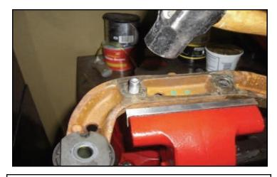
Remove the pressed in studs from the hanger. You can press them out or use a hammer to remove. Discard as they will not be reused.
