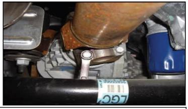
Mark the front driveshaft to pinion orientation for reassembly. Remove the front driveshaft from the differential and let hang out of the way.
