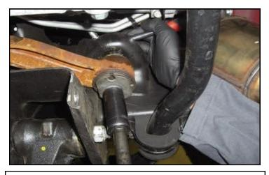
Remove the pass side differential hanger from the frame.
