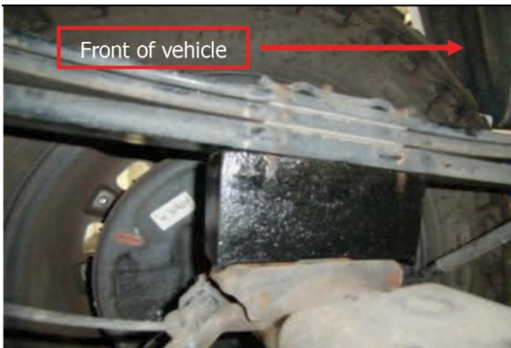
Tapered block with shorter end towards front of vehicle.
