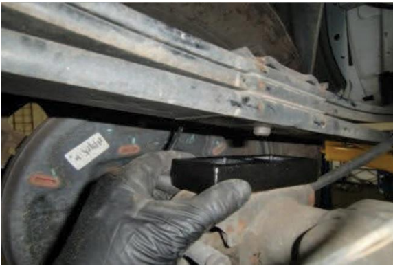
1" Blocks: Place new 1" block and take care that the pin is aligned with the hole in the block.
