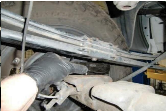
4WD Models; Remove factory block.
