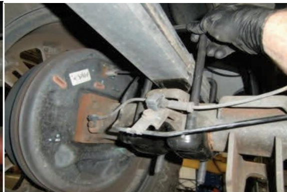
Remove U-bolt mounting hardware.
