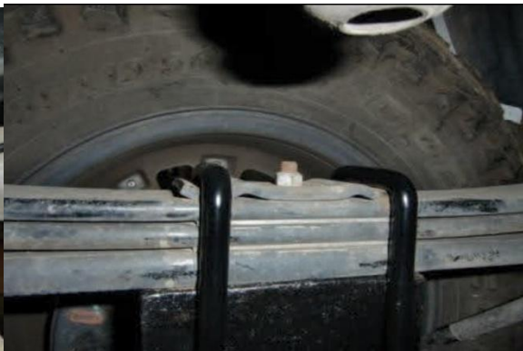
Make sure the top of the U-bolt is aligned in channels on upper plate.
