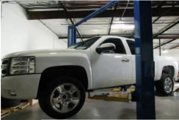
Raise and support vehicle by the frame.
