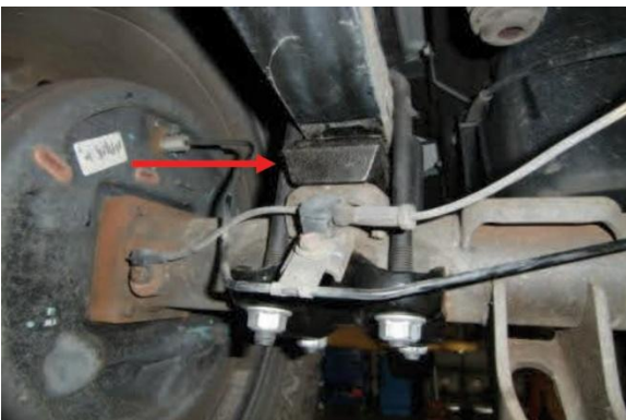
4WD models will have a factory block.
