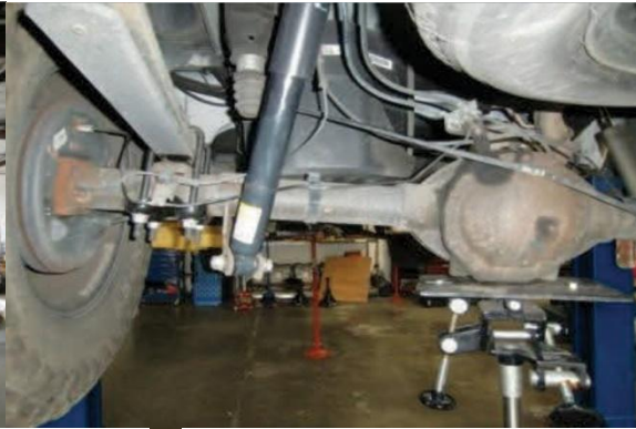
Support the rear axle with a jack.
