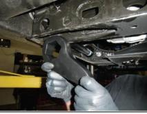
Adjust loading tool just enough to remove torsion key adjusting block from cross member. Release tool and remove.
