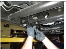
With torsion bar tool remove adjuster bolt.
