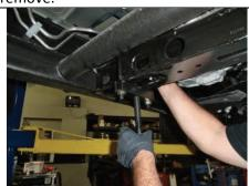
Use torsion bar loading tool and adjust new forged torsion key up just enough to allow adjuster block to be reinstalled.
