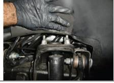
Note: To prevent damaging torsion bar tool. Peel back wheel well liner and remove (2) upper shock mounting nuts.
