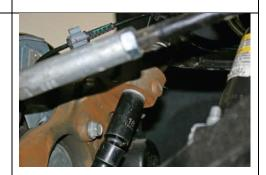
Tighten upper ball joint to spec.
