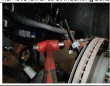
Carefully strike spindle as shown to separate ball joint.
