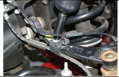
Disconnect ABS/brake bracket from upper control arm.
