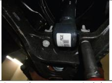
Remove lower strut mounting bolts
