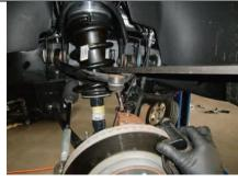
Lift suspension slightly while prying down to attach ball joint.
