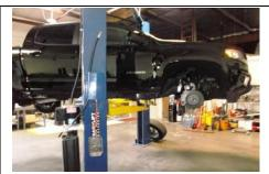
Lift the vehicle by the frame. Then remove the front wheels using a 22mm socket.
