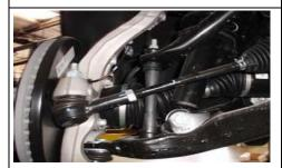
Reinstall the sway bar end links using a 13mm socket for the bottom.
