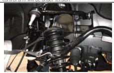
Lift the sway bar out of the way, then remove the strut
