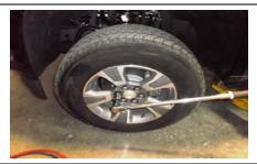
Reinstall the wheels using a 22mm socket, lower vehicle to the ground and torque the lug nuts to 100 ft lbs.
