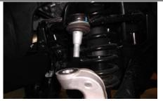
Separate the upper control arm from the steering knuckle using an 18mm socket. Note: the upper control arm will be upder topsion
