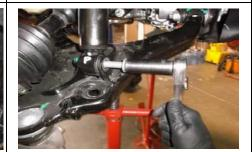
Raise the lower control arm and reinstall the bottom of the strut using a 21mm socket. Torque down.
