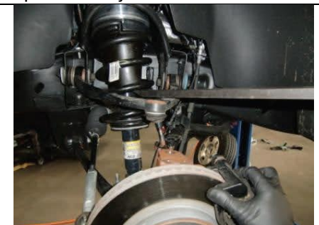
Carefully strike spindle as shown to separate ball joint.
