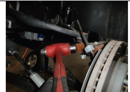
Carefully strike spindle as shown to separate ball joint.
