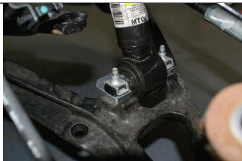
Loosen upper ball joint nut and leave attached.
