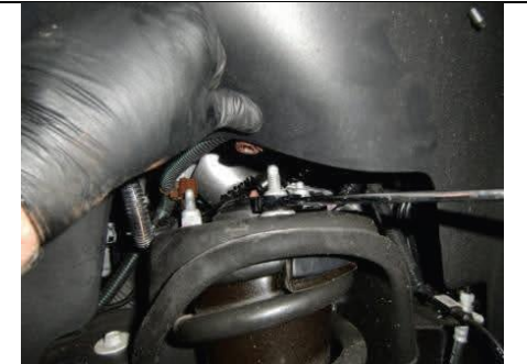
Loosen upper strut mount bolts
