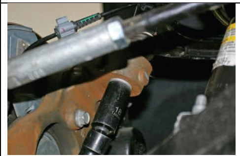
Tighten upper ball joint to spec.
