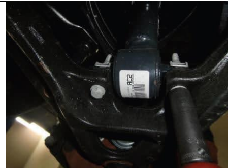
Remove lower strut mounting bolts
