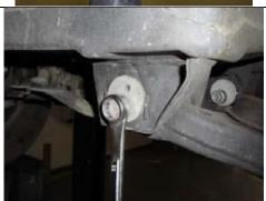
3 ) Rotate the lower control arm down.
