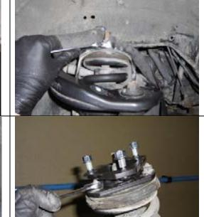
4 ) Rotate the strut 180 degrees and install onto vehicle. Install the supplied upper strut mounting nuts but leave them loose.
