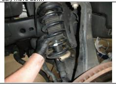
Push suspension down and remove strut from vehicle.
