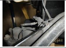
On backside of spindle remove ABS/brake line bracket
