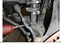
Remove lower strut mounting bolt/nut
