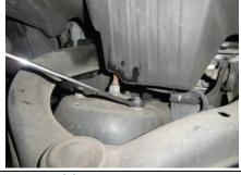
Remove (3) upper strut mounting nuts
