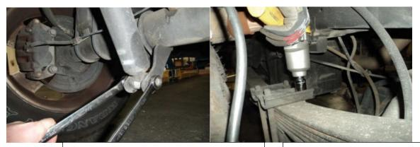
Remove the lower shock mount hardware.
