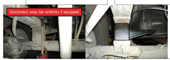
Remove U-bolts from axle and carefully lower the axle.
