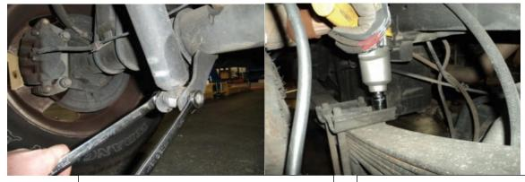
Remove the lower shock mount hardware.
