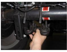
Remove u-bolt nuts and lower plate.
