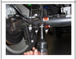
Loosen and remove factory u-bolt hardware.
