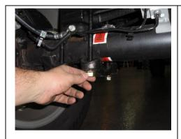
Attach lower mounting plate with provided hardware.
