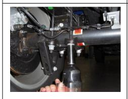
Loosen and remove factory u-bolt hardware.
