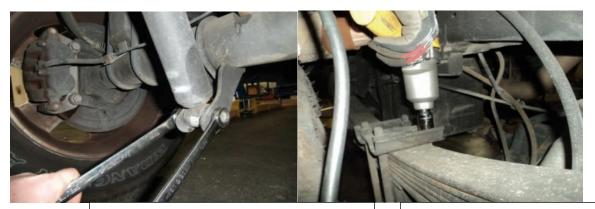
Remove the lower shock mount hardware.
