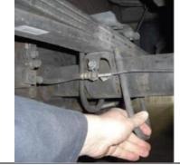
Remove u-bolts and carefully lower axle.
