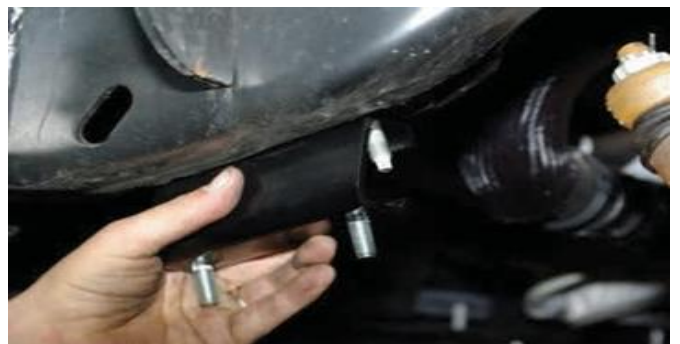
Install the sway bar drop bracket with factory hardware and torque to spec.
