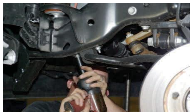
Remove factory sway bar bracket
