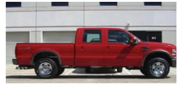
Place vehicle on level ground and measure ride height.
