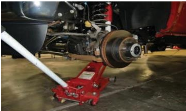
Support front axle with floor jack(s).
