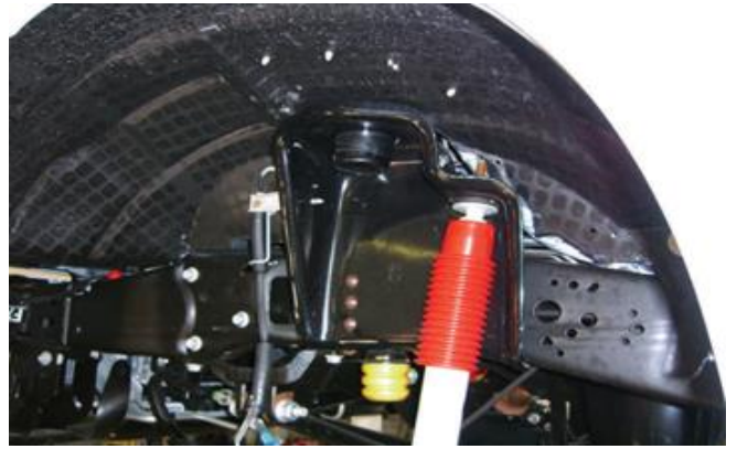
Carefully lower front axle and remove front coil springs.
