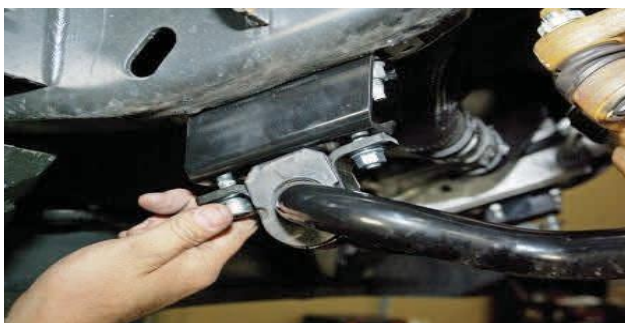
Reattached Sway bar to drop bracket using factory hardware
