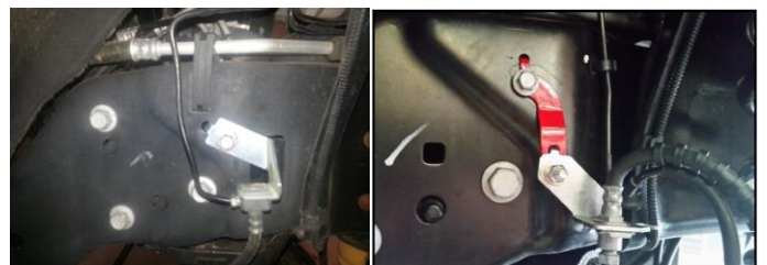
05-08 Drill a 3/8" hole 1.5" lower on the frame rail and secure brake line with original bolt. 2010-17 Reinstall brake line brackets, driver on pass side, pass on driver side. Loosen the hard line ferrule and rotate 180 degrees and retighten. Re-attach brake line block to bracket with factory clips.
