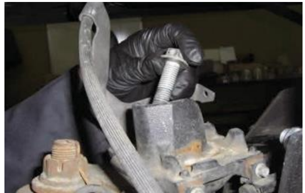
Remove bolt from the spring perch
